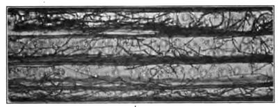
Fig. 35.—Thin section of rotting pine showing fungous threads and holes where these have penetrated through the walls of the wood cells.
